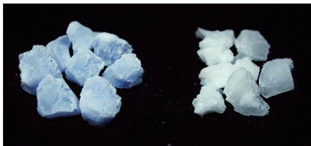
Figure 1. Lumps of an \text{O}_3 + \text{O}_2 + \text{CO}_2 hydrate (left) and an \text{O}_2 + \text{CO}_2 hydrate (right). Each lump is about 5 mm in linear dimension. The pale blue color of the \text{O}_3 + \text{O}_2 + \text{CO}_2 hydrate lumps had faded somewhat during their short exposure to the room air before the picture was taken owing to icing on their surfaces, but their color is still distinguishable from the milk-white color of the \text{O}_2 + \text{CO}_2 hydrate lumps.
